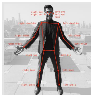
Fig. 1. Seventeen pose key points detected by posenet[6]
